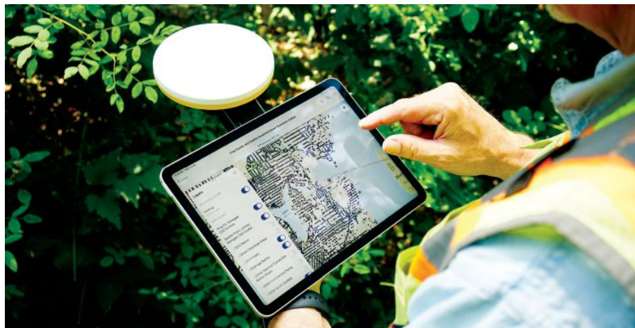
Cost-effective positioning is available for any industry by turning a smartphone or tablet into a precision mapping, navigation, and measurement tool with Trimble Catalyst, a GNSS concept delivering positioning-as-a-service to Android and iOS devices.
