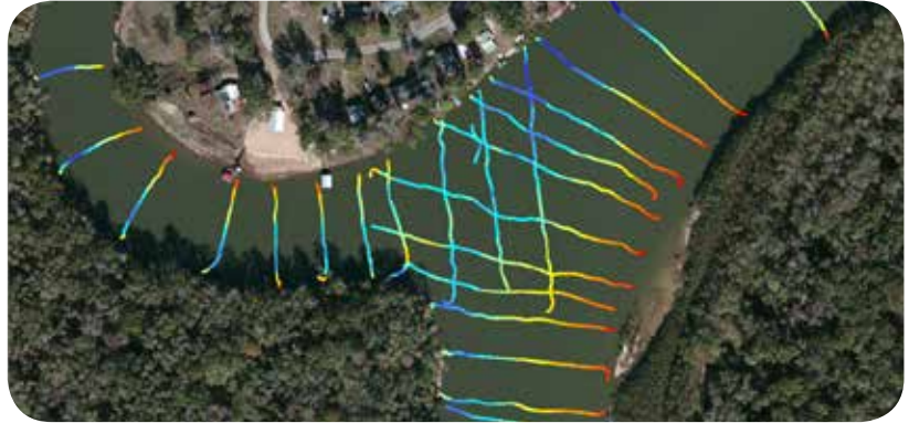
Bathymetric image using single beam echosounder. Image provided by CBEC Engineering, Inc.
