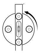
Make minor adjustments with leveling screws if necessary.
