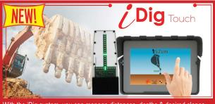
With the iDig system, you can manage distances, depths & desired slopes. The combination of advanced technologies is unique in the world: no cables, radio communication, simplified installation & solar charging!
