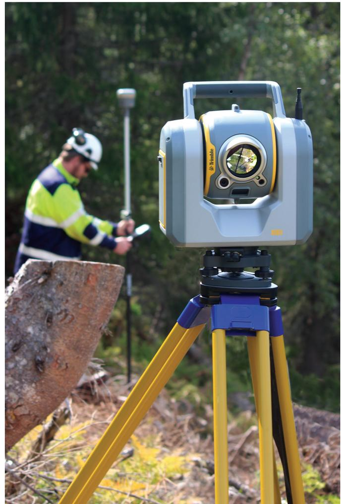
*The Geomatikk team used the Trimble R10 and the SX10 to establish ground control.*
