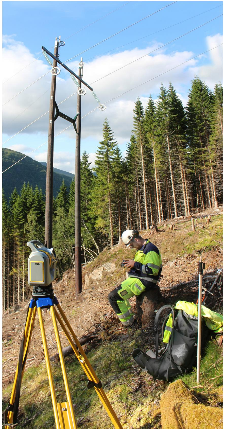
*The Geomatikk crew acquired two scans of the power lines. Here the SX10 scans from the bottom of the slope while Even Sellevoll monitors the controller.*
