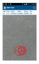
You then have to orientate your device so that the two crosshairs become concentric and green in color, meaning the TDC650 device is leveled. Then gently move the device horizontally so that the
