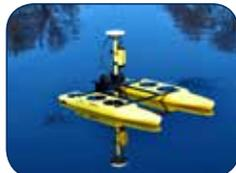
HydroLite-TM mounted on HyDrone-RCV
